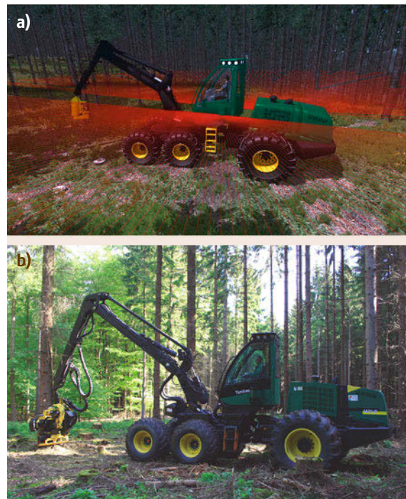
Fig. 56.24 (a) A simulated wood harvester equipped with simulated laser scanners in a virtual testbed used for algorithm development and evaluation. (b) The physical harvester in the woods, equipped with laser scanners mounted to the right and left door of the cabin
