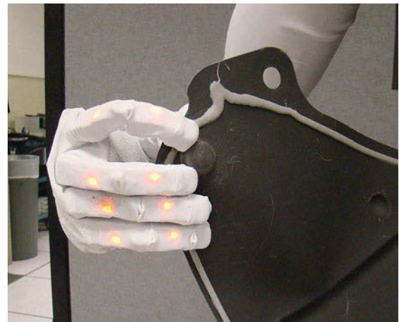
Fig. 41.14 Robot exploring a 2-D deformable object (after [41.59])
