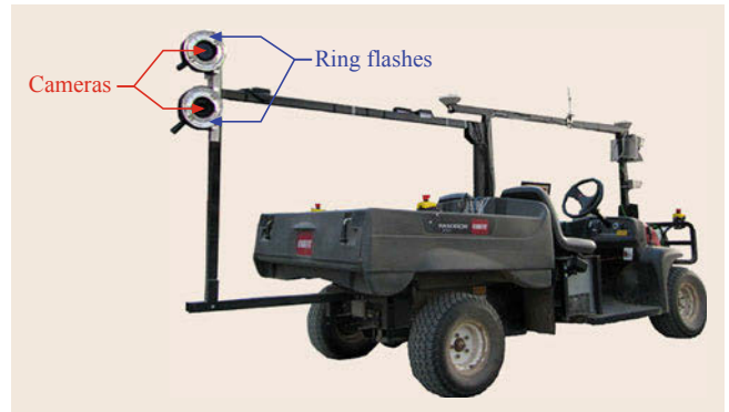
Fig. 56.8 Autonomous crop yield estimation system hardware, composed of concentric cameras and ring flashes for controlled illumination during nighttime operations
