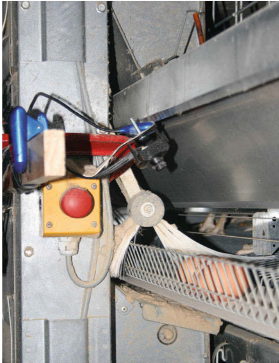
Fig. 56.33 Prototype computer vision system for scanning the egg collection belt for potential blockages
