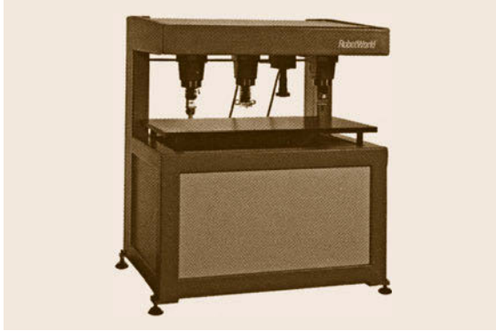
Fig. 4.13 RobotWorld is an integrated workcell with multiple robot modules that move on air bearings
