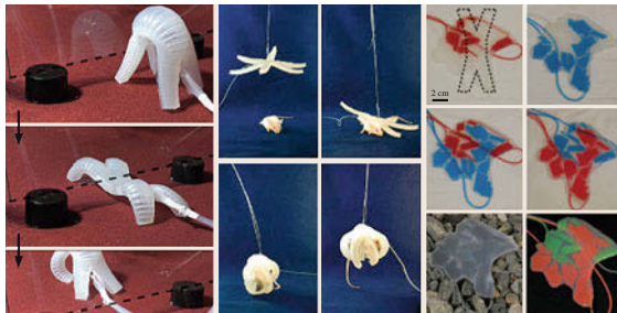
Fig. 23.40 Bio-inspired soft robots and actuators manufactured by soft lithography (after [23.130, 131, 135, 136])
