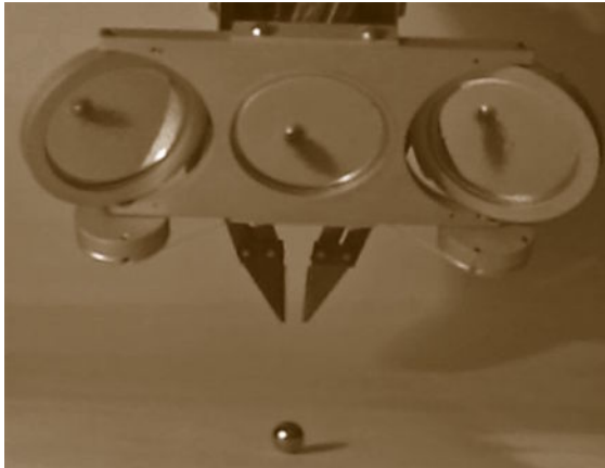
Fig. 30.28 Biomimetic configuration sonar with center transmitter flanked by receivers that rotate
