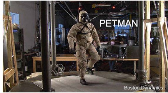
Fig. 67.7 Petman is a humanoid robot that Boston Dynamics developed to test chemical protection clothing for the US military (after [67.26])
