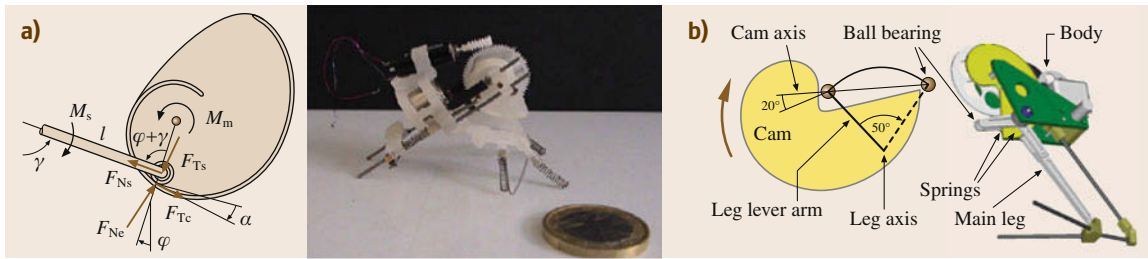
Fig.23.16a,b Escapement cam mechanism (a) Grillo (Ver.1) (after [23.86]) and (b) 7 g jumping robot (after [23.87])
