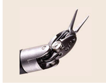
Fig. 4.14 Wrist for surgery has no singularities within range of motion. Features tungsten cable actuation (after [4.49])
