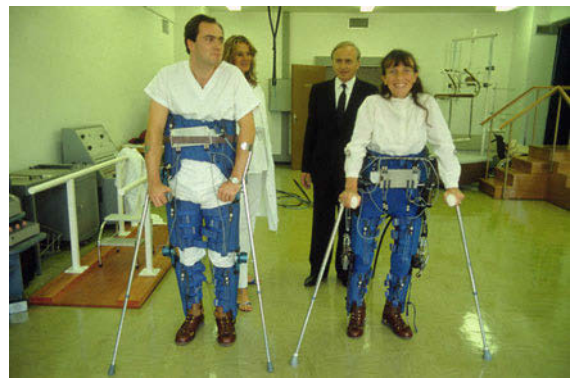
Fig. 64.2 This machine developed by Professor Rabischong allows the patient in rehabilitation to maintain her balance while inciting her muscles to move (after [64.47])
