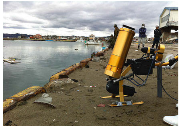
Fig. 58.22 Underwater reconnaissance robot being evaluated in search for human remains following the March tsunami, Japan. (courtesy of Prof. Shigeo Hirose)
