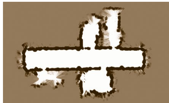
Fig. 45.3 Occupancy grid map obtained from ultrasound data (after [45.2])
