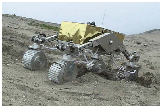
Fig. 50.2 Lateral- and side-slip situation of wheeled mobile robot
