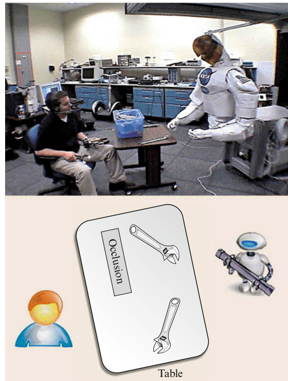
Fig. 72.6 Robonaut using visual perspective taking to disambiguate the intended referent when asked to hand me the wrench . The human can only see one wrench, but the robot can see both. The robot correctly hands the wrench that both can see
