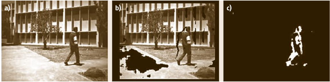
Fig. 31.23a–c Independent motion detection from a moving platform. Reference image on panel (a) is forward-projected using the motion homography to the image on panel (b); image on panel (c) is the difference with the actual image
