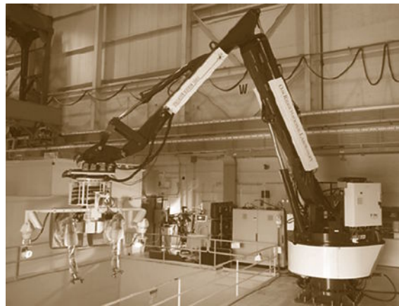
Fig. 58.20 SNS pedestal manipulator system
