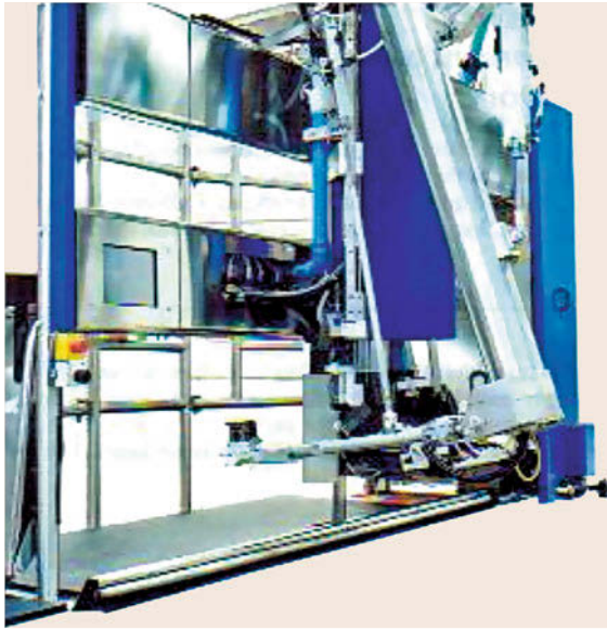
Fig. 4.12 DeLaval Cow Milking System features hydraulic robot with machine vision guided positioning (VIDEO 643)
