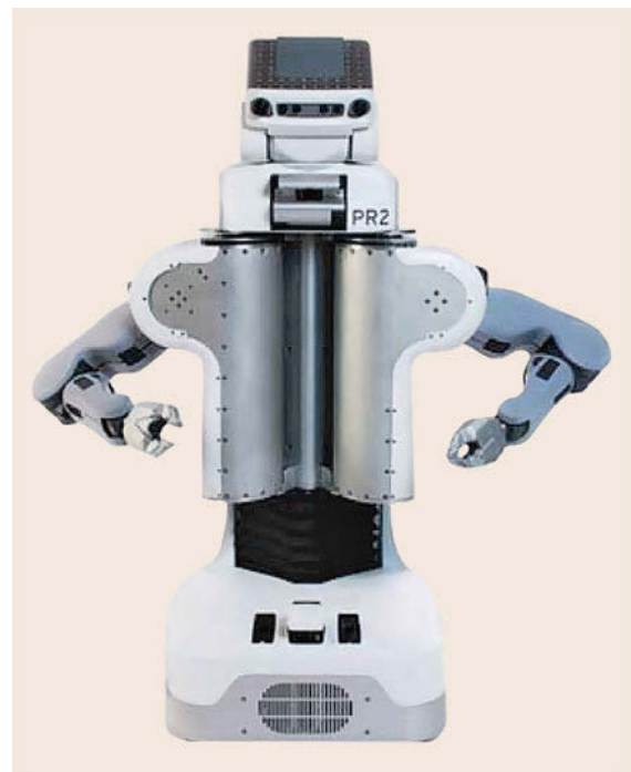
Fig. 17.16 PR2 robot from Willow Garage using springs for passive gravity compensation (after [17.22, 23])
