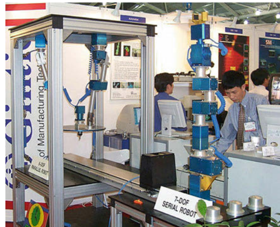
Fig. 22.2 15-axis Reconfigurable Robotic Workcell (after [22.9])
