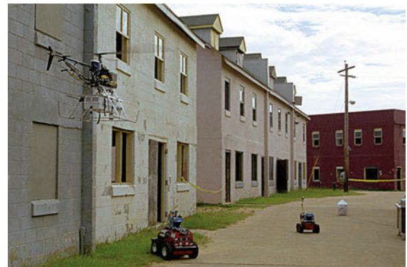
Fig. 53.14 Heterogeneous team of an air and two ground vehicles that can perform cooperative reconnaissance and surveillance
