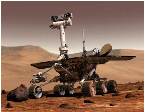
Fig. 55.20 The Mars exploration rovers, Spirit and Opportunity, with a manipulator arm in front
