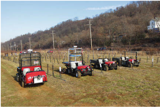
Fig. 56.11 A family of autonomous orchard vehicles capable of driving among tree rows, based on the Toro Workman series. To keep cost low, the vehicles use only a laser rangefinder and steering and wheel encoder for perception and navigation
