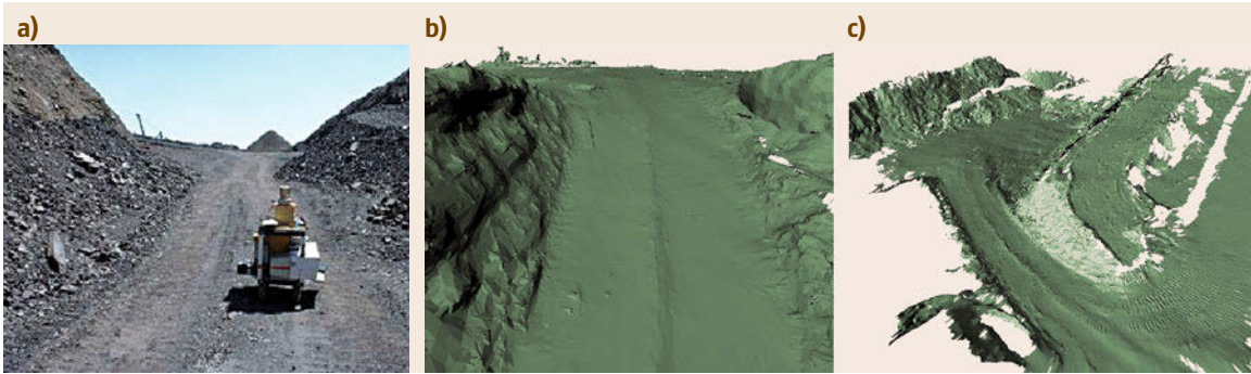
Fig.45.15a-c Two views (b-c) of the mesh representation of a map (a) obtained by scanning an environment. The meshes are reduced by a factor of 10 from the initial data
