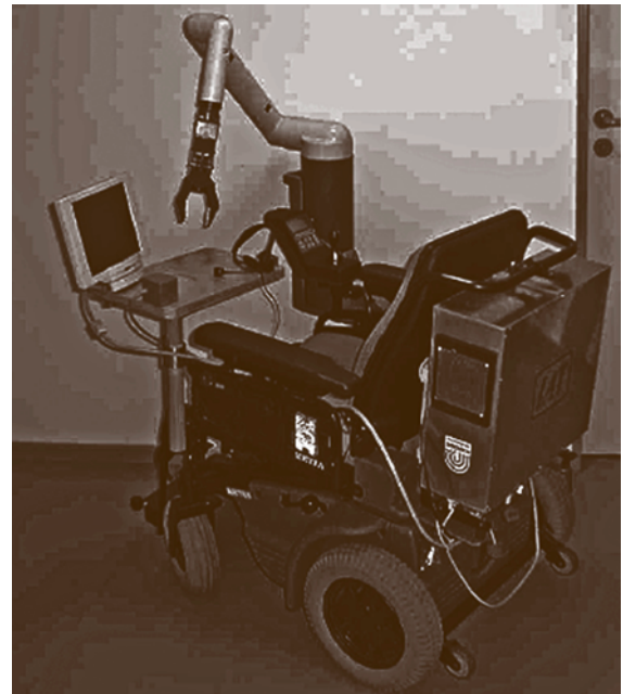
Fig. 64.13 Wheelchair manipulator robot MANUS developed at the Rehabilitation R&D Center, Hoensbroek, and marketed by Exact Dynamics (The Netherlands)
