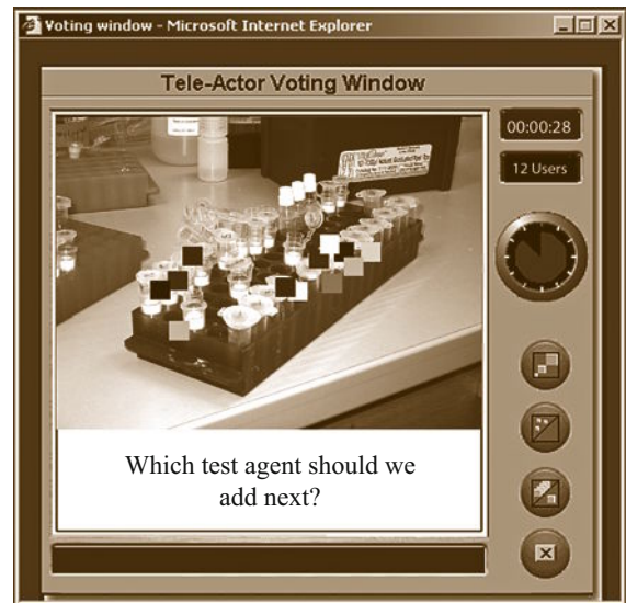
Fig. 44.11 Spatial dynamic voting interface for the Tele-Actor system: the spatial dynamic voting (SDV) interface as viewed by each user. In the remote environment, the Tele-Actor takes images with a digital camera, which are transmitted over the network and displayed to all participants with a relevant question. With a mouse click, each user places a color-coded marker (a votel or voting element) on the image. Users view the position of all votels and can change their votel positions based on the group's response. Votel positions are then processed to identify a consensus region in the voting image that is sent back to the Tele-Actor. In this manner, the group collaborates to guide the actions of the Tele-Actor (after [44.53])
