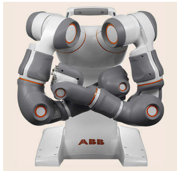
Fig. 10.7 A cooperating dual-arm concept robot by Asea Brown Boveri (ABB)
