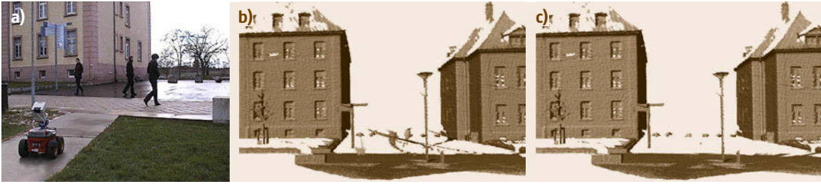
Fig. 45.21 (a) A mobile robot acquiring a three-dimensional scan of an urban scene. (b) The people in the scene cause spurious data points in the resulting meshes. (c) The same scene after filtering people
