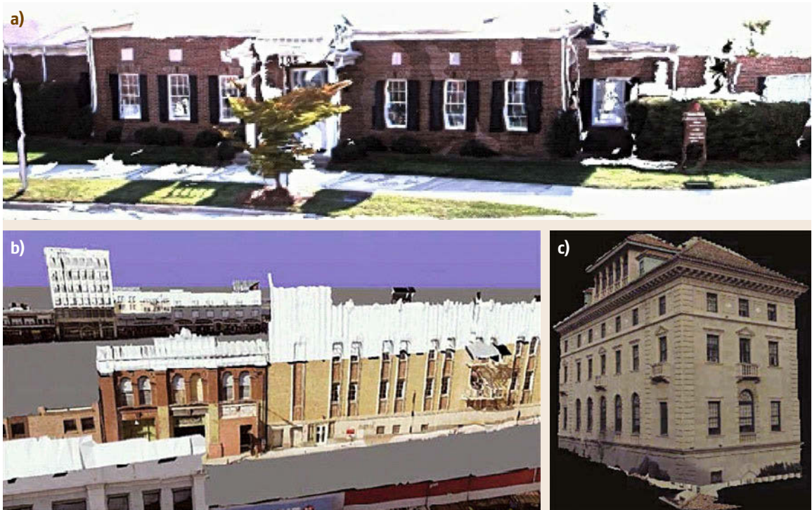
Fig.45.16a–c Examples of urban terrain modeled as a textured mesh (a) (after [45.35]), (b) (after [45.37]), and (c) (after [45.36])
