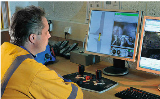
Fig. 59.14 Teleoperator's station for control of underground robotic vehicles at the Kemi mine, Finland (courtesy of Atlas Copco, 2009)
