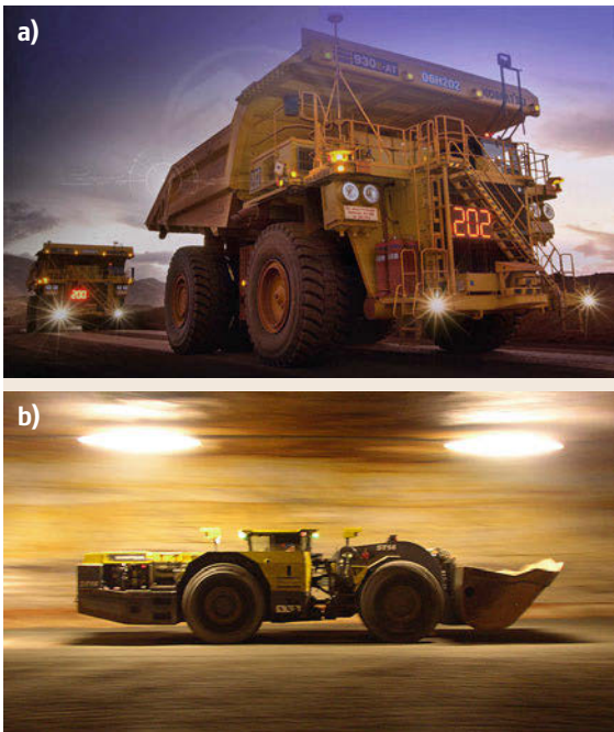
Fig. 59.1 (a) Examples of robotic vehicles in underground and surface mining. Unmanned surface haul trucks (Photo: Mobular Mining Systems, 2011); (b) an autonomous underground load-haul-dump (LHD) machine at the Kvarntorp mine, Sweden (Photo: Joshua Marshall, 2007)
