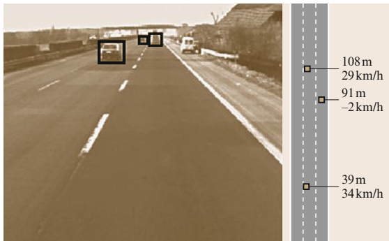
Fig. 62.11 Vehicle detection – lane and range position
