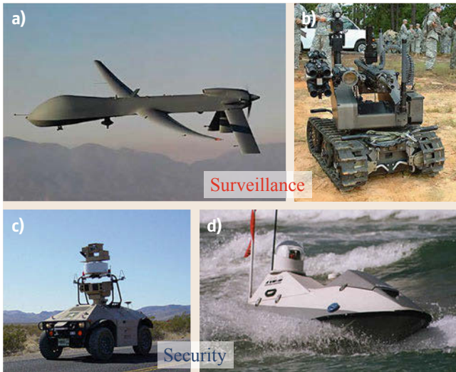
Fig. 61.1a–d Examples of surveillance and security robots. (a) Aerial-General Atomics Predator, (b) ground-QinetiQ TALON, (c) ground-General Dynamics MDARS-E, and (d) surface water-Elbit Stingray
