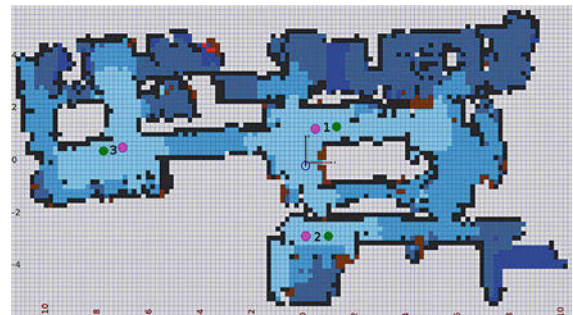
Fig. 65.18 Robot map obtained with vector field SLAM in a 125 m 2 home environment
