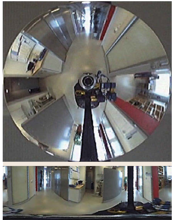
Fig. 5.10 Catadioptric image and the same image mapped to a cylindrical surface
