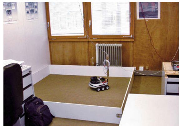
Fig. 76.16 A mobile robot with a pan-tilt camera is asked to move within the walled arena in the office environment
