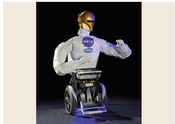
Fig. 67.12 The NASA (National Aeronautics and Space Administration) Robonaut consists of an upper body placed on a wheeled mobile base
