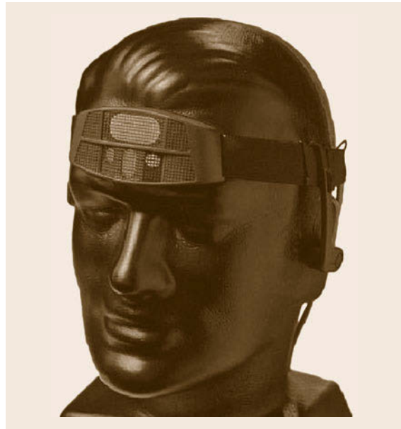
Fig. 30.22 Aid for blind people – the small oval transducer is the transmitter and the other three components are receivers. The large oval receiver provides high resolution, enabling fixation by users' fine neck control (after Kay [30.58])
