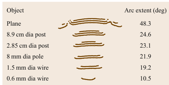
Fig. 30.15 PAS sonar maps of six objects located at 1 m range. The sonar is located below the objects in the figure
