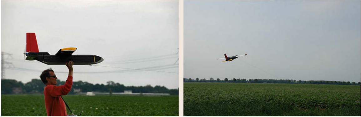
Fig. 56.38 Operator launching an unmanned aircraft over a potato field via a launch rope. The plane then flies autonomously following a pre-programmed flight path
