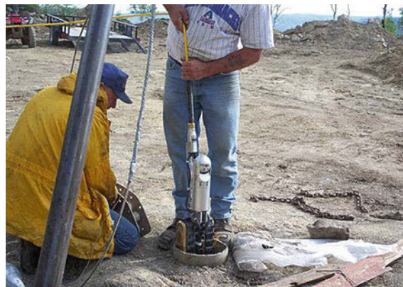
Fig. 60.10 The Inuktun mine crawler robot being lowered into a borehole at the Crandall Canyon mine (courtesy of CRASAR)
