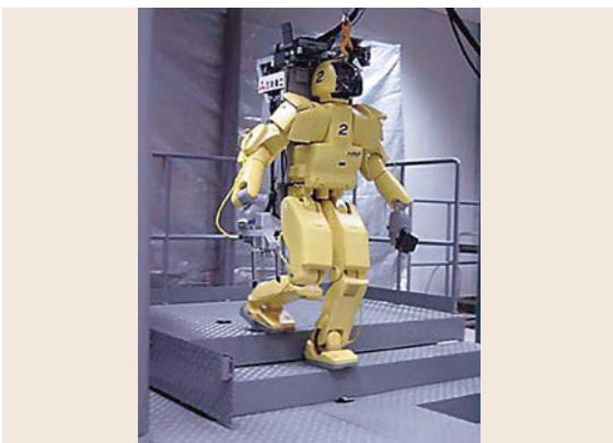
Fig. 67.2 HRP-1 operating in a mockup of an industrial plant (courtesy Mitsubishi Heavy Industries)
