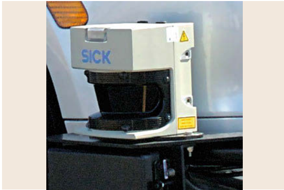
Fig. 5.8 Example laser ranging sensor (SICK LMS291) that is widely used in mobile robotics
