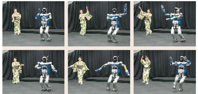
Fig. 67.4 The humanoid robot HRP-2 dancing with a human (after [67.25]). The human is a master of a traditional Japanese dance whose dancing was recorded by a motion-capture system, and transformed for use by the robot
