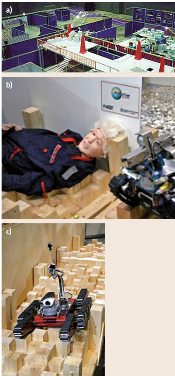
Fig. 60.18a–c View of the NIST standard test bed for search and rescue used by RoboCup Rescue. (a) View of overall test bed, (b) dummy representing a victim, and (c) a step field challenging robot mobility (courtesy NIST )
