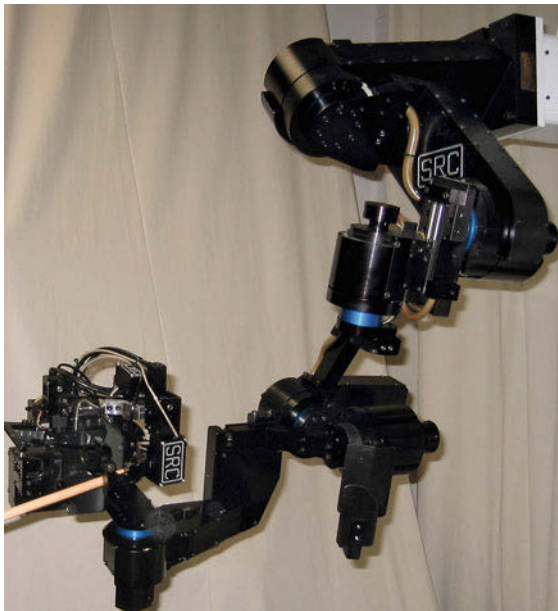
Fig. 15.5 The 7 degree of freedom anthropomorphic SAR-COS arm used in learning inverse dynamics, inverse kinematics, and operational space control
