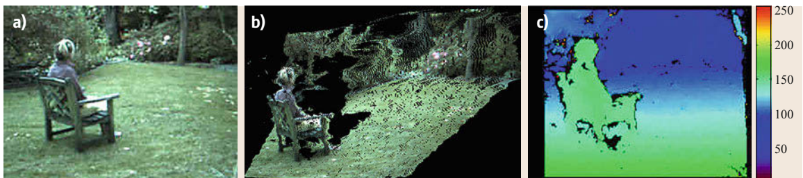
Fig. 31.10a–c Sample stereo results from an outdoor garden scene; baseline is 9 cm. (a) original left image. (b) computed 3-D points from a different angle. (c) disparity in pseudo-color
