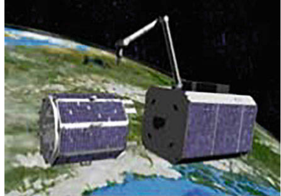
Fig. 55.13 DEOS – orbital servicing experiment with client (left) and servicer (right)
