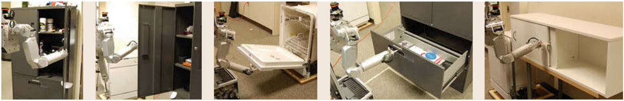
Fig. 41.12 Robot manipulating a variety of common articulated objects (from left to right): a cabinet door that opens to the right, a cabinet door that opens to the left, a dishwasher, a drawer, and a sliding cabinet door (after [41.55])
