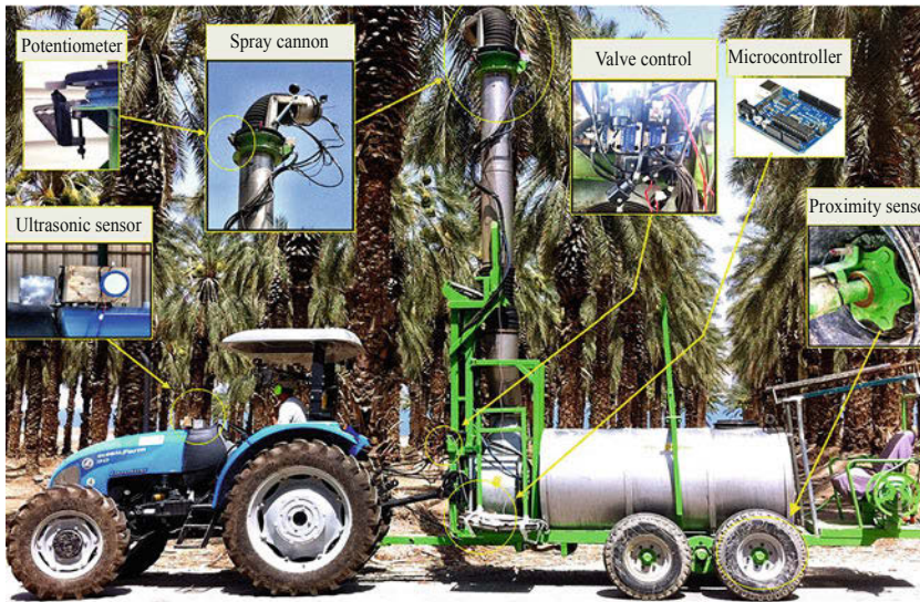
Fig. 56.14 Date tree tracking system adapted to a commercial sprayer. The system aims the sprayer nozzle toward the trees more efficiently and safely than a human operator
