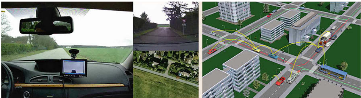
Fig. 62.16 A collision warning system for intersection safety implemented on communicating Renault experimental vehicles using the intention/expectation approach (after [62.26])
