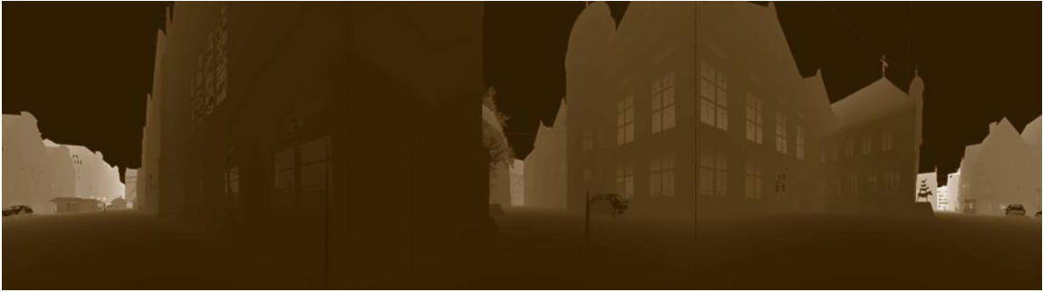
Fig. 31.4 3-D range scan represented with three rectilinear projections (Fig. 31.1)
