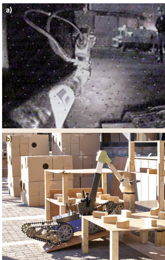
Fig.60.17a,b Examples of tracked robots with manipulator arms that have been used for disasters or rescue competitions. (a) View from Foster-Miller Talon at the WTC of its arm (courtesy of CRASAR ) and (b) teleMAX by Telerob at the Rescue Robotics Camp (courtesy of R. Sheh)
