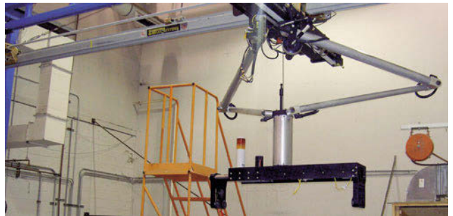
Fig. 11.13 A large flexible linking arm with command shaping
