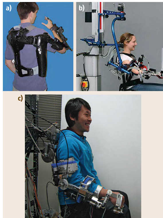
Fig.70.2a–c Upper limb exoskeletons for the shoulder–elbow–wrist complex: (a) RUPERT (after [70.14]); (b) ARMIN (after [70.15]); (c) SUEFUL-7 (after [70.16])
