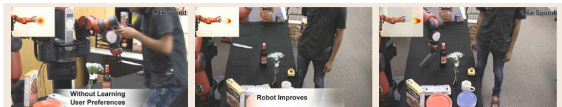
Fig. 69.18 The robot Baxter learns to safely handle a knife ([69.130]; courtesy of Saxena's Robot Learning Lab)
