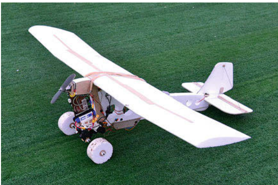
Fig. 52.7 An autonomous fixed-wing aerial robot for experimental work on vision-based terrain tracking at ANU (after [52.41]). Note the upswept wings to generate dihedral and the lack of ailerons
