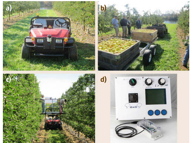
Fig. 56.12 (a) Autonomous orchard vehicle. (b) Workers on foot harvest apples and deposit them on bins towed by the vehicle, eliminating the need for and the cost of a tractor driver. (c) In this version the vehicle is equipped with a lift platform from where workers can prune, thin, tie trees, and place pheromone dispensers up to twice as fast as workers performing the same operations on ladders. Users on the platform control the vehicle from an interface (d) that communicates with the onboard computer wirelessly
