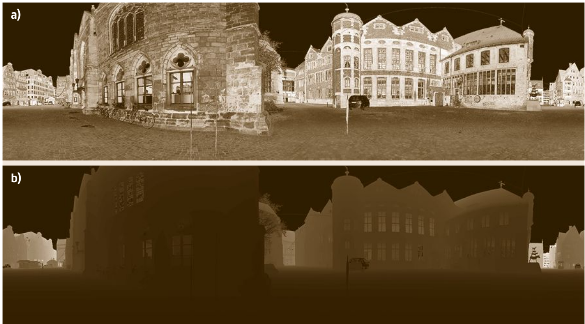
Fig. 31.1a,b 3-D laser scan with a field of view of 360^\circ \times 100^\circ acquired in an urban environment (Bremen downtown). (a) Registered infrared reflectance image. (b) Range image where closer is darker
