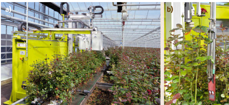
Fig. 56.20a,b A rose harvesting robot. (a) The robot with the rose crop on a mobile growing system. (b) The end-effector with stereo vision system and a scissors-type cutting device (courtesy Jentjens Machinetechniek BV, Veghel, The Netherlands)
