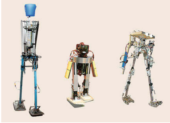
Fig. 67.18 These robots from Delft, MIT and Cornell (left to right) are designed to exploit their natural dynamics when walking (after [67.57]; courtesy Steven H. Collins)
