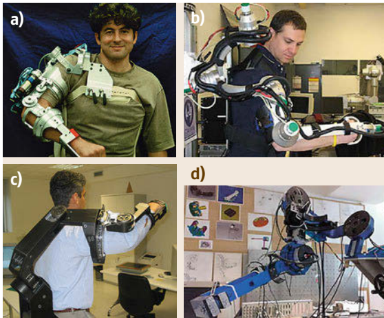
Fig.70.3a–d Upper limb exoskeletons for the shoulder–elbow–forearm complex: (a) PERCRO-I (after [70.34]); (b) MGA (after [70.19]); (c) PERCRO-III (after [70.9]); (d) RehabExos (after [70.20])
