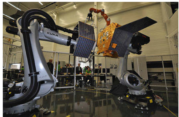
Fig. 55.35 OOS-SIM, a hardware-in-the-loop simulator in DLR
