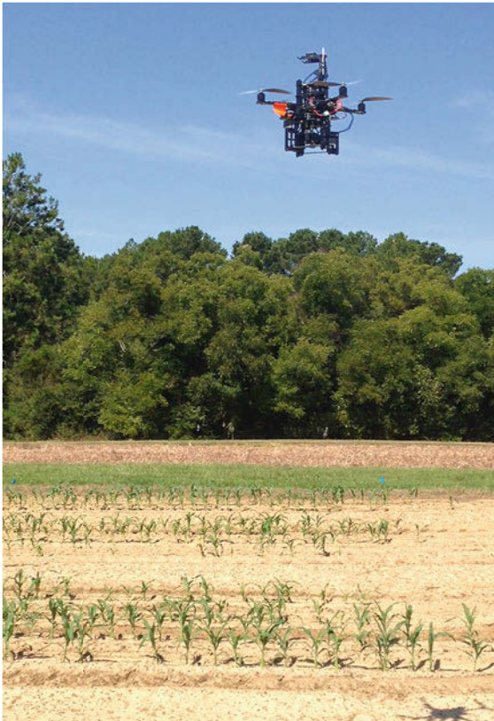
Fig. 56.36 AscTec Pelican quadrotor used for data collection over early season sweet corn
