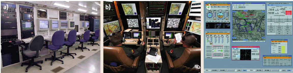
Fig. 61.8a–c Global Hawk ground elements: (a) ground station, (b) operator seats, and (c) UAV display (courtesy of Northrop Grumman and Raytheon)
