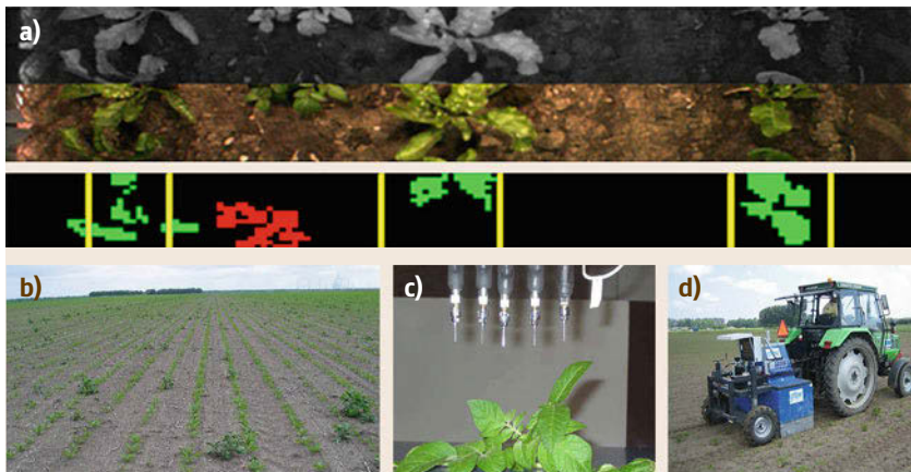
Fig. 56.5a–d Precision removal of volunteer potatoes in sugar beets. (a) Computer vision-based detection of the potato weeds (red) among the sugar beet plants (green). (b) A sugar beet field infested with potato weeds. (c) A micro-spray system. (d) The removal device pulled by a tractor
