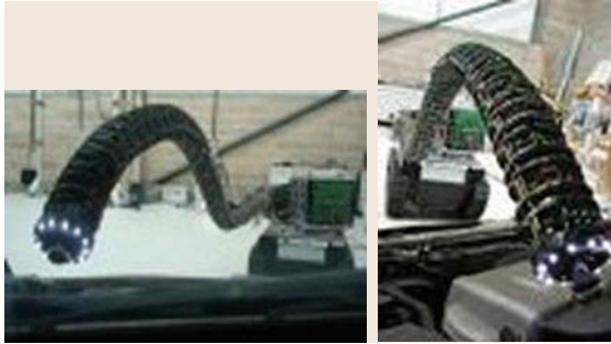
Fig. 20.12 The OC Robotics Snake-Arm robot – an externally actuated continuum-like robot with segmented backbone (after [20.75])
