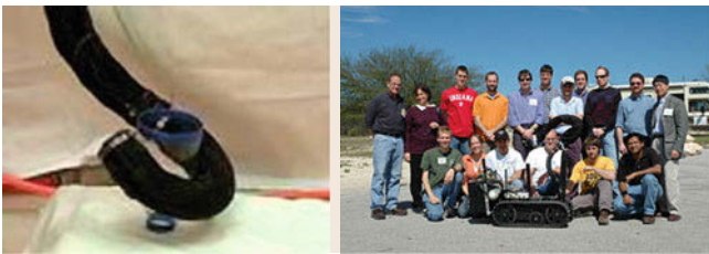
Fig. 20.13 The intrinsically actuated Octarm pneumatic continuum manipulator and its development team (after [20.42])
