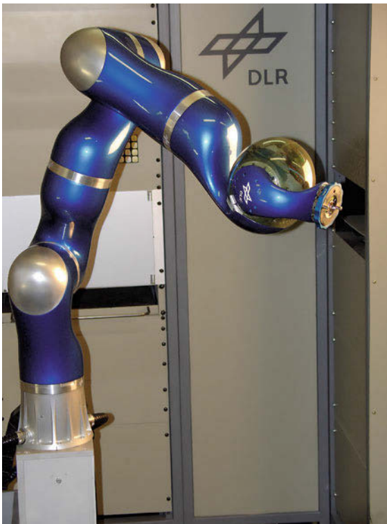
Fig. 11.3 The lightweight manipulator DLR LWR-III by the German Aerospace Center
