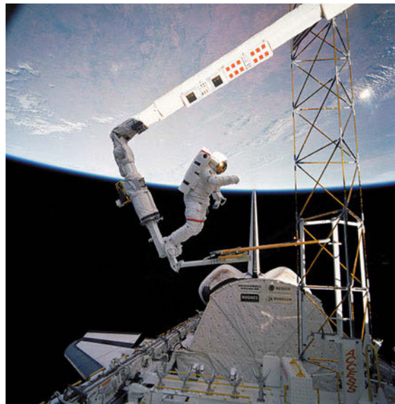
Fig. 55.3 Space shuttle remote manipulator system (SRMS) used as a platform for an astronaut's extra vehicular activity in the shuttle cargo bay
