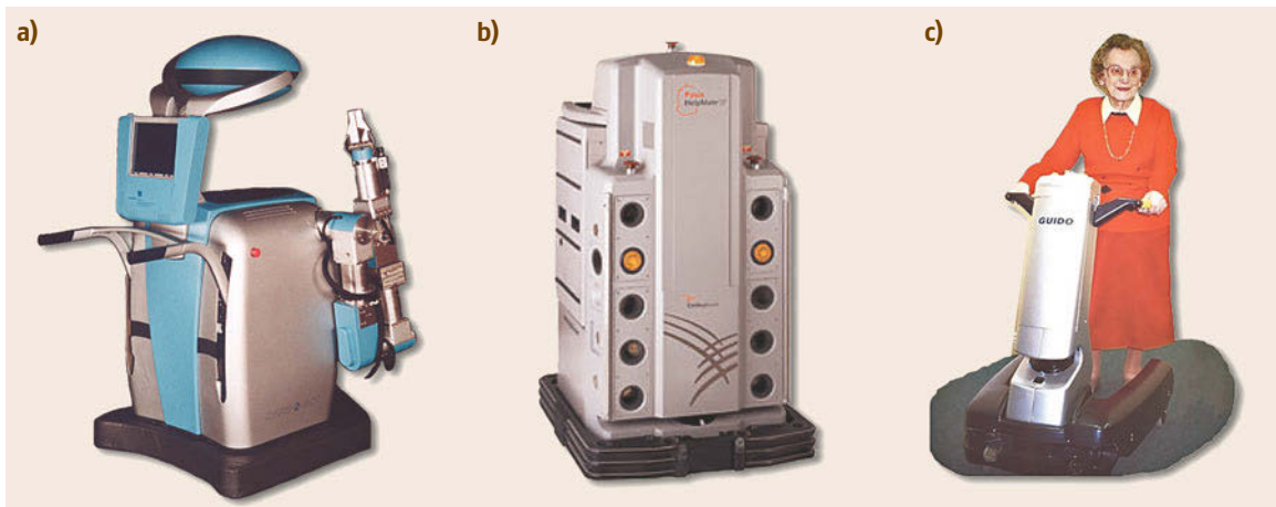
Fig.64.16a–c Human assistance robots: (a) Care-O-bot, developed by the Fraunhofer Research Institute (Germany). (b) Helpmate by Transitions Research Inc., USA. (c) Pam-Aid (aka Guido), developed in the UK
