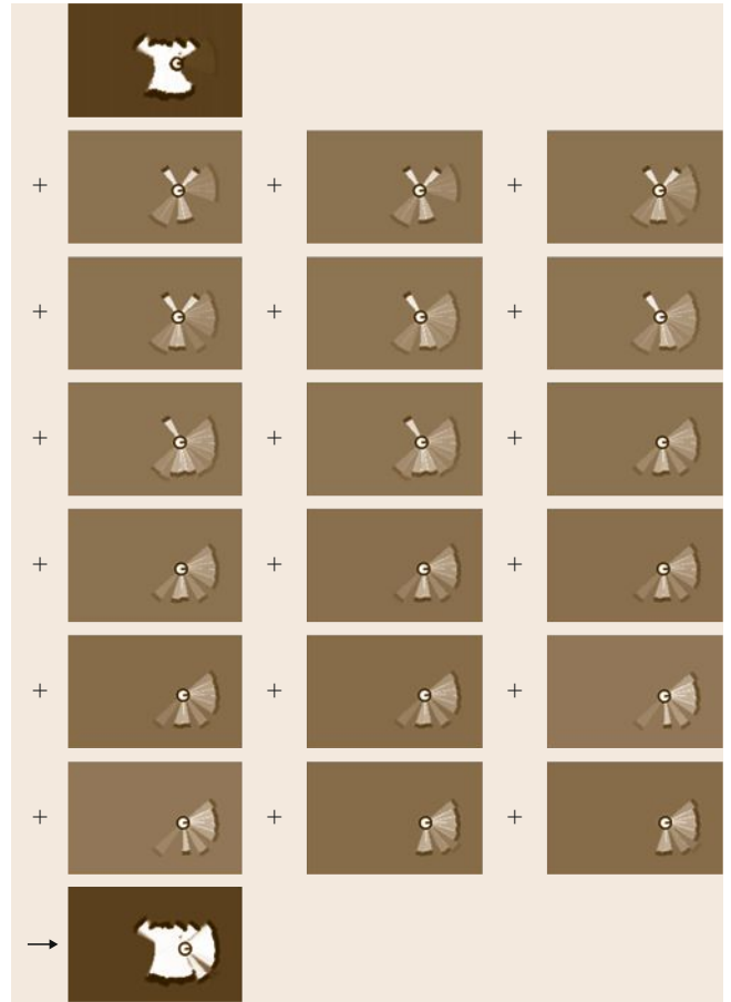
Fig. 45.2 Incremental mapping in a corridor environment. The upper left image shows the initial map and the lower one shows the resulting map. The maps in between are the local maps built from the individual ultrasound scans perceived by the robot (after [45.2])
