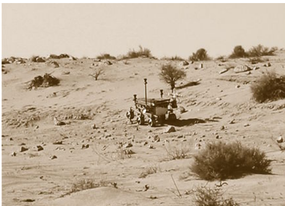
Fig. 50.3 Rocky 8: rocker-bogie configuration with six steerable wheels robot
