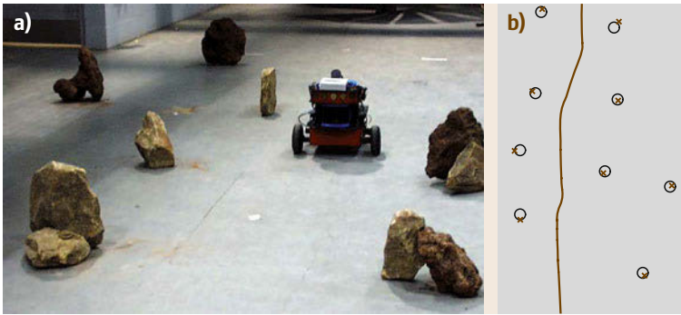
Fig. 45.7 (a) Mobile robot mapping a set of stone rocks. The image (b) depicts the path and the estimated landmark positions. The manually determined positions of the rocks are marked by circles (after [45.6])
