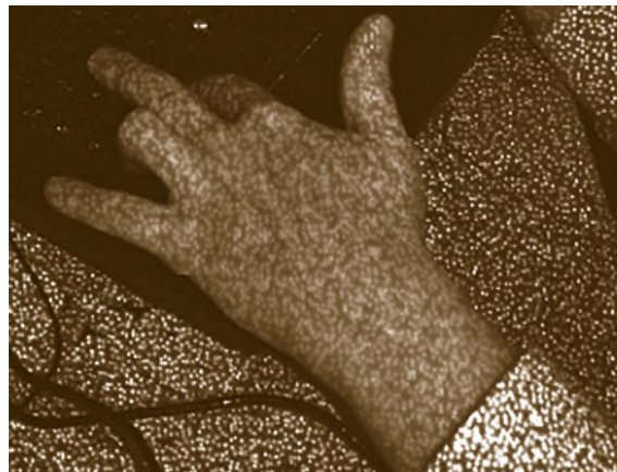
Fig. 31.11 The laser grid of the Kinect for calculating depth
