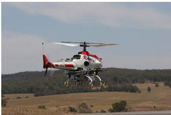
Fig. 52.1 Autonomous aerial robotic vehicle based on the Yamaha RMAX platform developed in the University of New South Wales, Australia (after [52.3, 4])
