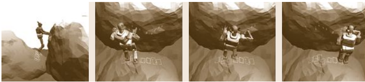
Fig. 67.37 A sequence of planned whole-body motion including multiple contacts on a irregular terrain (after [67.108])
