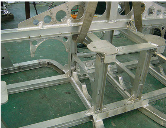
Fig. 25.1 Aluminum frame of an ROV, Hamire, developed by KRISO, Korea
