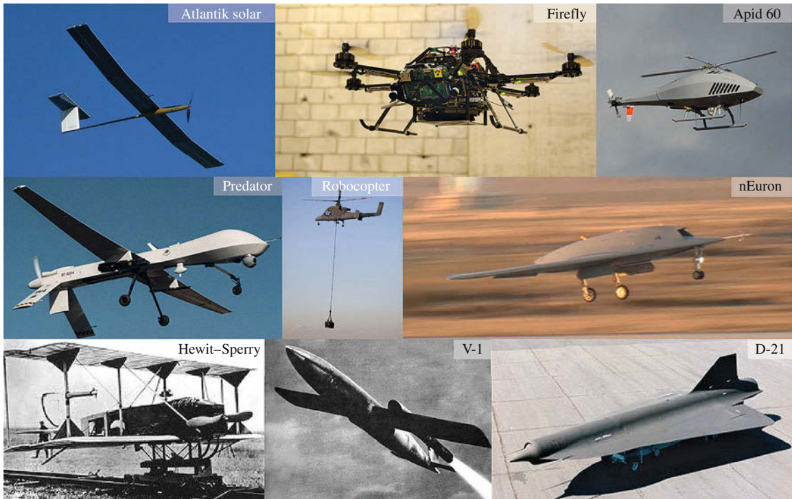
Fig. 26.1 A glimpse on the UAS history through some examples starting from the Hewitt–Sperry Automatic Airplane (1917), the V-1 flying bomb (1944), and the Lockheed D-21 (1962) until the recent examples of military (Predator, Robocopter, nEuron) and civilian (AtlantikSolar, Firefly, Apid 60) aerial robots
